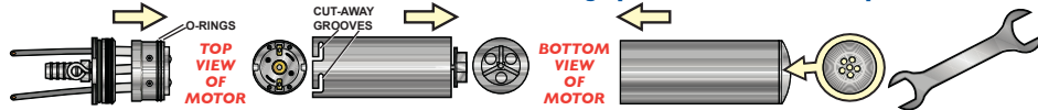
Fig. A - The motor housing top connector Fig. B - The replaceable motor module Fig. C - The outside pump housing. Fig. D - The ProActive Wrench
